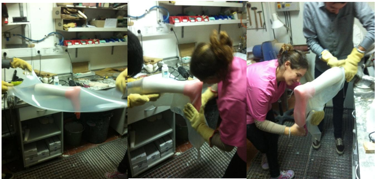
Fig. 34 - (a) placement the polypropylene in positive cast, (b) molding of material and (c) cut off excess material
