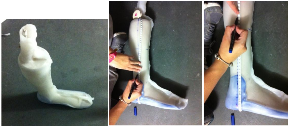
Fig. 35 - (a) Material molded on the plaster cast, (b, c) drawing of the sagittal line on the molded material
