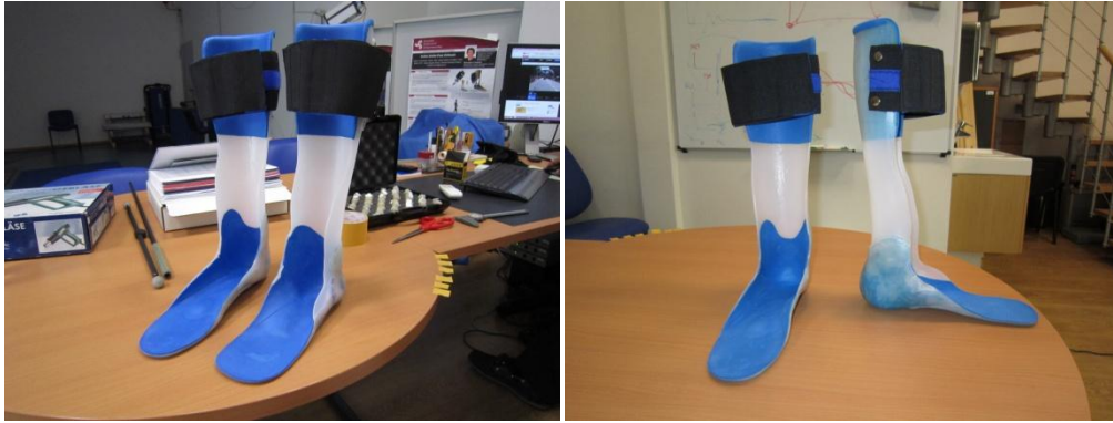
Fig. 38 - AFOs ready for trial (a) frontal plan, (b) frontal plan right side and sagittal plan left side
